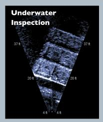
This image shows the bottom side of a floating dock at close range. The dock's structure and features are clearly visible in even the murkiest conditions.
